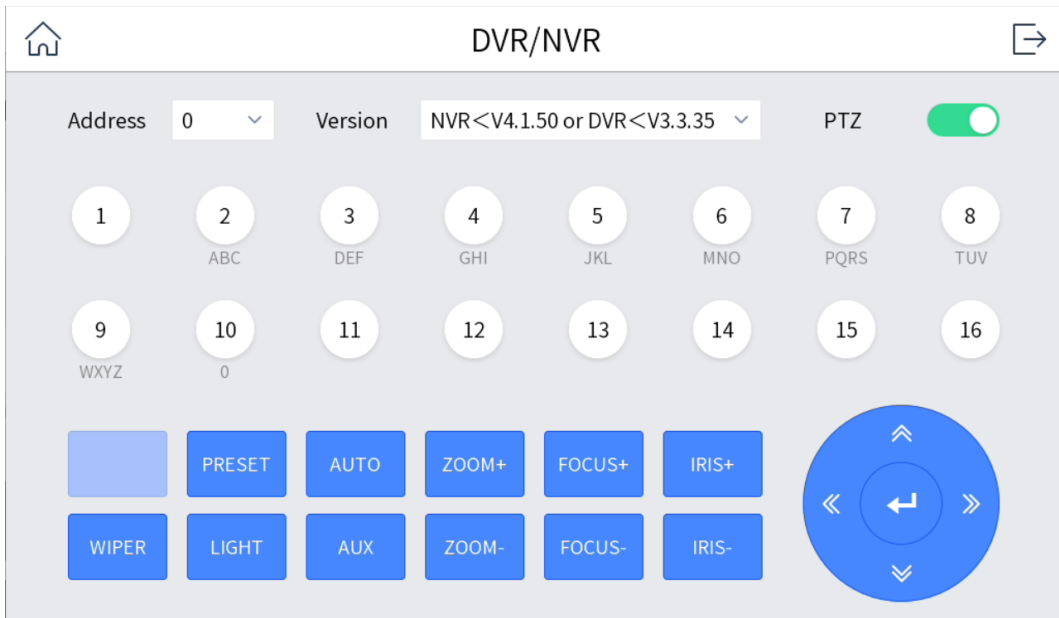
Figure 4-23 Connect Video Recorder (PTZ Enabled)
